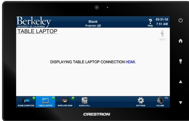
1. Press “WIRELESS HDMI” icon from home menu or toolbar to display content from your device using wireless HDMI presenter on the projection screen.
